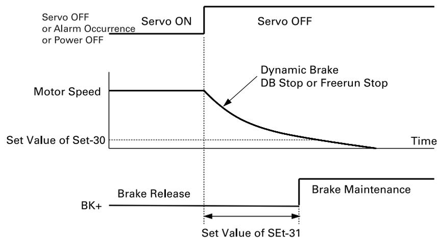
The brake signal will be produced if the motor speed is smaller than the set value of the parameter or the time set at SEt-31 passed after the servo is OFF.
