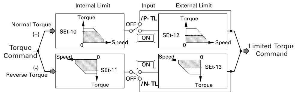
/P-TL signal is used to externally limit the forward torque, and /N-TL signal is used to externally limit the reverse torque. These external torque limits have priority over internal torque limits. Internal limits are used to restrain the maximum value of the motor's operating torque (or output torque) within a fixed range so that the load system or operation targets can be protected.
