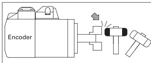
Excessive impact during coupling assembly can damage the encoder.
