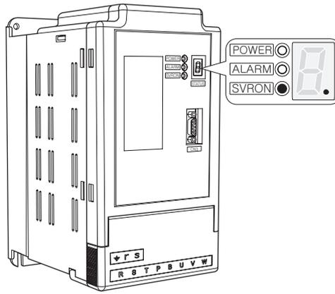
When the Servo is ON, a dot will be lit. And SVRON light will be on.
