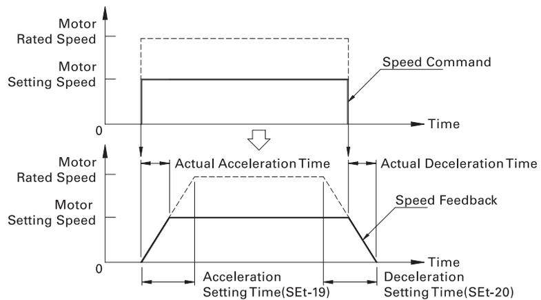
The diagram shows that the time for execution compared to command got extended as much as the deceleration time.
