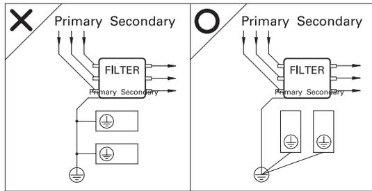
Connect the grounding line of the noise filter to the grounding frame separately. Please do not connect the grounding line of the noise filter to other grounding lines.
