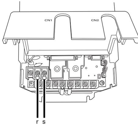
Connect the single-phase voltage to r and s terminals to supply power to the control circuit.
