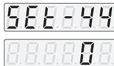
Please determine whether to maintain the dynamic brake function after the motor has stopped on the second digit of SEt-44.
