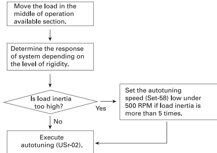
If it is set too low compared to the load, the calculated inertia ratio can be inaccurate.
