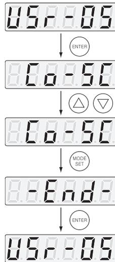
Manual adjustment for speed command offset should be done when the servo is ON.
