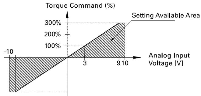
If the torque command gain is 100%/3V and the input voltage is 9 V, 300% torque, the maximum torque of the motor, will be generated.
