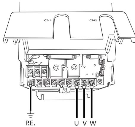
Connect the motor power supply cable to U, V, and W terminals.
