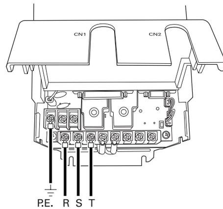
Connect the 3-phase voltage to R, S, and T terminals to supply power to the main system.
