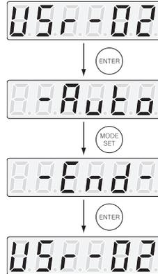
During the process of auto tuning, the following parameter will be automatically set.
