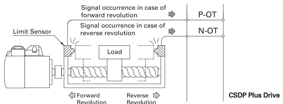
The overtravel signal is not the servo alarm but a signal to protect the load system.
