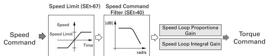
Raising the speed loop proportional gain can improve the response of the speed control loop. Please set the value as high as possible within a range that won't cause vibration.
