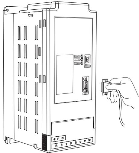
Connect the operator cable to CN3 (9 pin) terminal.
