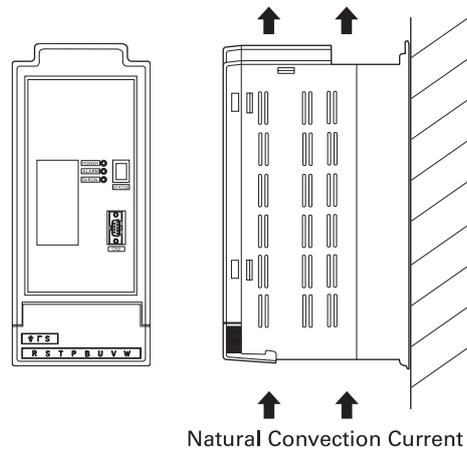
Please make sure that the drive is installed vertically for enhanced cooling efficiency.
