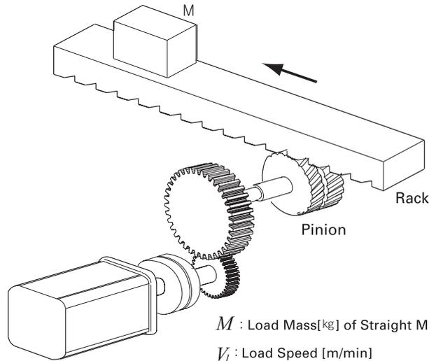
$M$  : Load Mass[kg] of Straight Movement Part     $F$  : Thrust [N]
