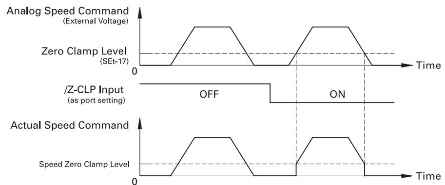
If the CN1 connector pins where the zero clamp function is allocated are ON, the voltage command below the level set at SEt-17 will be ignored. When the value of the speed command surpasses this level again, the motor will be accelerated to the value of the command.
