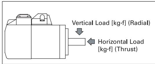
Please make sure the load on the motor shaft doesn't exceed load allowance. Please refer to the motor specifications in the appendix for the allowed load for each motor.
