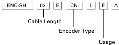
Write 1H5 to order a 1.5 m-long cable, 05 for a 5m-long cable, and 40 for a 40 m-long cable. Write CL if a 15-wire Abs type encoder is needed, CL for a 11-wire Inc type, and CH for a 17-bit Serial type encoder. Write F for a cable to fix up and M for a flexible cable.
