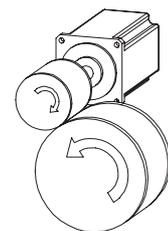
The speed reduction ratio is the ratio of revolutions of the system to the motor. If the system make one revolution when the motor makes five revolutions, the speed reduction ratio is 5. If the system make five revolutions when the motor revolves once, then the speed reduction ratio is 0.2.
