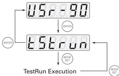
Pilot operation will be repeated in the same pattern until it is aborted. The 1 cycle is 14 seconds.
