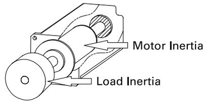
In tuning, the inertia ratio should be considered first for the optimum performance of the servo drive system. The inertia ratio is the ratio of the inertia of the load to the that of the motor's rotor. If the rotor's inertia is  $3 \text{ gf.cm.s}^2$  and the load's inertia is  $30 \text{ gf.cm.s}^2$ , the inertia ratio is 10.
