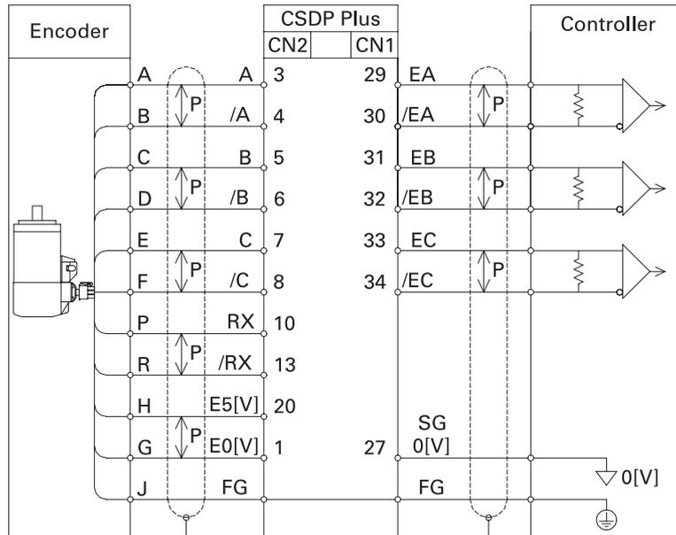
**11-wire Incremental Encoder Wiring**
