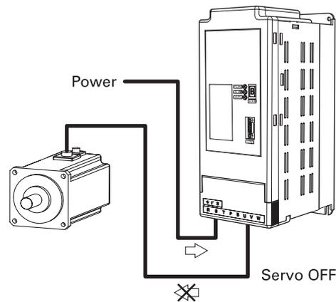
If the power supply is engaged but servo-ON signal is not issued, the servo drive and the motor are separated.
