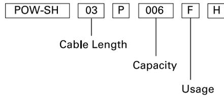
Write 1H5 to order a 1.5 m-long cable, 05 for a 5 m-long cable, and 40 for a 40 m-long cable. If 1.5 kw capacity is required, write 015.
