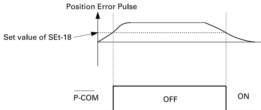
If this parameter is high in the low-speed operation, the position completion signal can be kept ON. This signal can usually be used as a reference signal for the next sequence of the operation.
