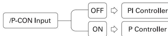
Therefore, at the controller, a program to shift the speed controller from PI controller type to P controller type can be made by assessing the analogue output such as the speed of the servo drive and torque and the output like /P-COM, /V-COM, /TG-ON.
