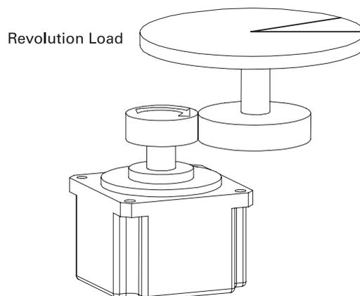
If the distance to move with one pulse of the controller is  $0.1^\circ$ , the denominator is 3600.
