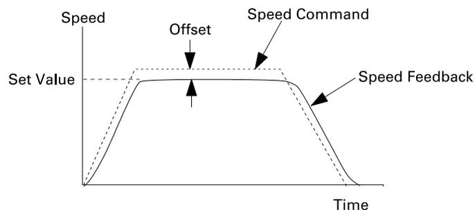
The integral value will be automatically adjusted based on the set value of the speed command. There can be speed offset if the speed exceeds the set value.
