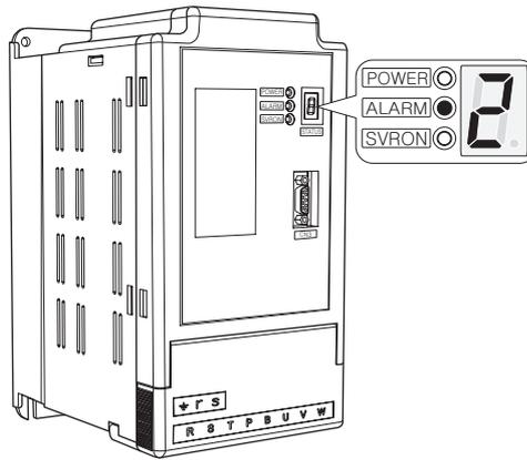
If an alarm occurs, the first digit of the relevant number will be displayed. And the ALARM light will be on.
