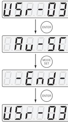
Auto adjustment for speed command offset can be done when the servo is either ON or OFF.
