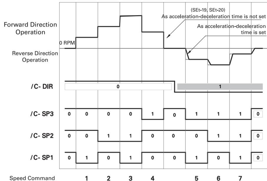
Set the acceleration time and deceleration time within the range that won't undermine the response of the system in order to ease the impact of speed change.
