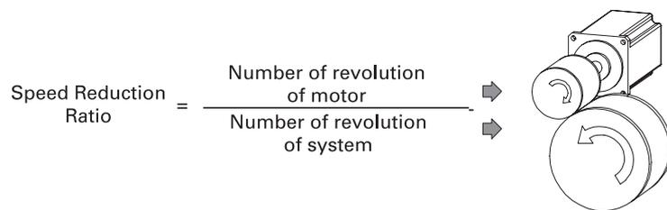
The speed reduction ratio is the ratio of revolutions of the system to the motor. If the system make one revolution when the motor makes five revolutions, the speed reduction ratio is 5. If the system make five revolutions when the motor revolves once, then the speed reduction ratio is 0.2.
