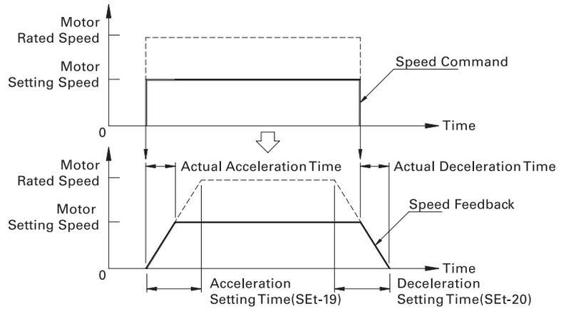
The diagram shows that the time for execution compared to command was extended as much as the deceleration time.
