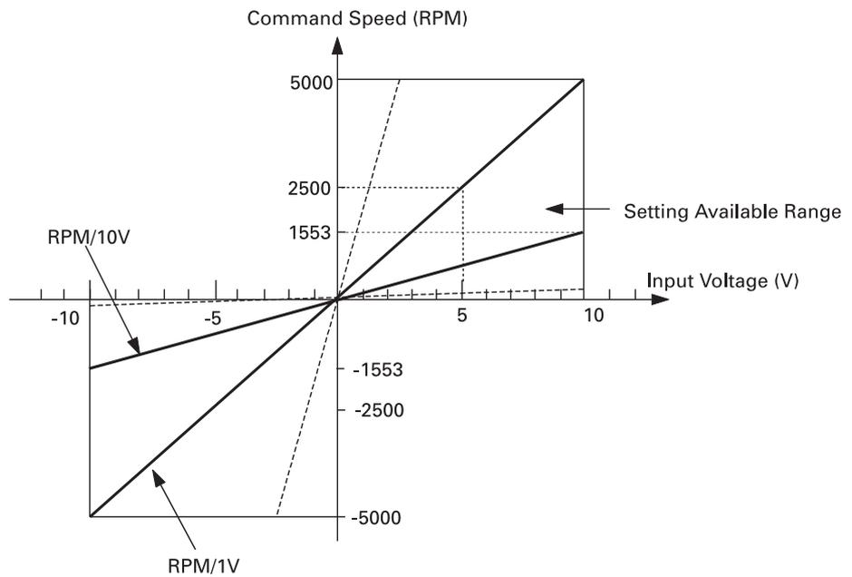
Speed command gain determines the gradient of the graph.
