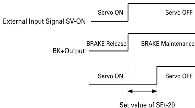
The parameter switches on the BK signal if the servo OFF signal is received when the motor stops, maintains the servo ON status internally for the time set at SEt-29 from the moment it receives the servo OFF signal, and switches the servo OFF after the preset time is passed.
