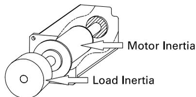
In tuning, the inertia ratio should be considered first for the optimum performance of the motor connected to the servo drive. The inertia ratio is the ratio of the inertia of the load to that of the motor's rotor.
