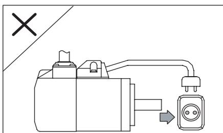
Please do not directly connect the motor to the power supply.
