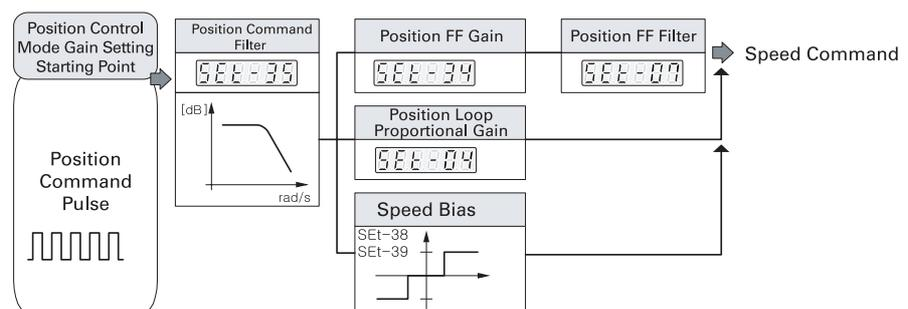
Position command filter can restrain the high frequency element in the position command to soften the position command itself. If its value is 0, position command filter will not be used.
