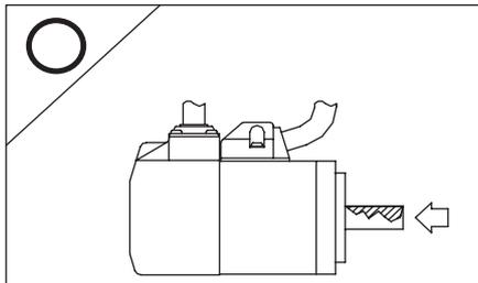
The shaft is oiled for corrosion prevention. Please remove it before installation.
