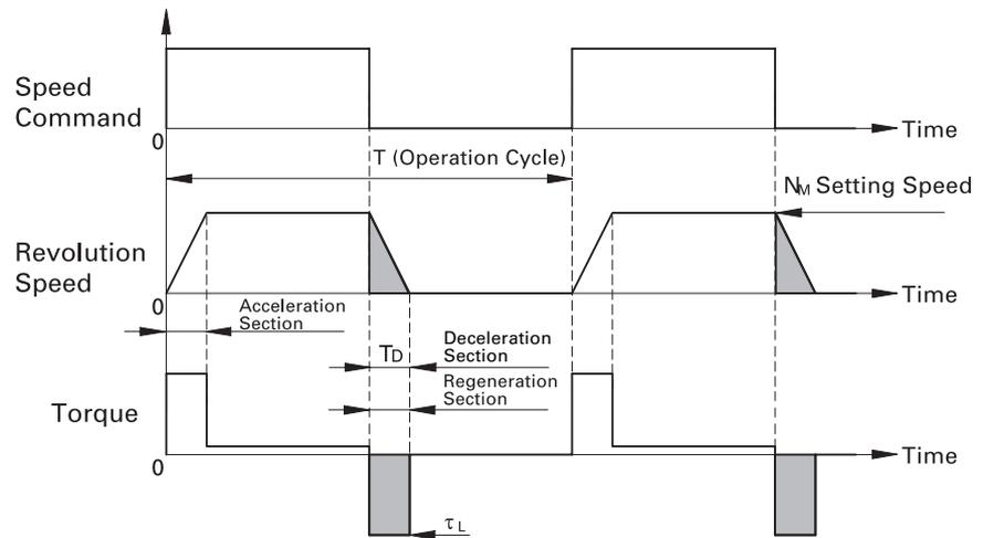
$$\text{Number of Repetition} = \frac{1}{T} \times 60 \text{ cycles/min}$$
