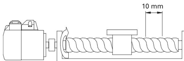
The ball screw finishes one revolution with 1000 pulses and thus a ball screw with 10 mm pitch can move 10  $\mu\text{m}$  with one pulse command.
