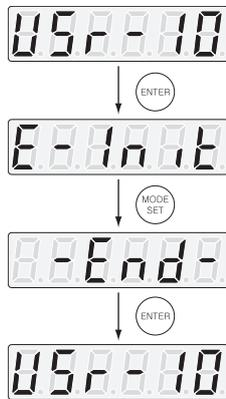
When an alarm occurs, the alarm code will be recorded in the order of PAr-01 to PAr-10. If USr-10 is implemented, all the values from PAr-01 to PAr-10 will be changed to 0.
