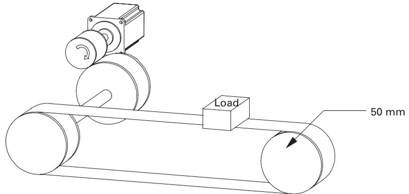
If the diameter of the pulley on the load side is 50 mm and the distance to move by one pulse of the controller is 100  $\mu\text{m}$ , the denominator is 1570.
