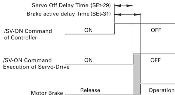
On the contrary, if the servo OFF delay time is longer than the brake active delay time, the brake on the motor starts working before the servo OFF is completed as shown below, preventing the fall of the vertical load.
