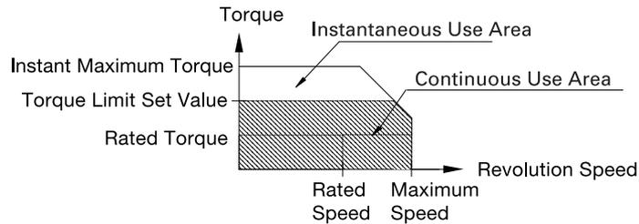
Depending on the type of a motor, Instantaneous maximum torque can be 300% or less. If the torque limit is set higher than the maximum allowed torque of the motor, the limit will be set at the Instantaneous maximum torque of the motor and the preset limit will be ignored.
