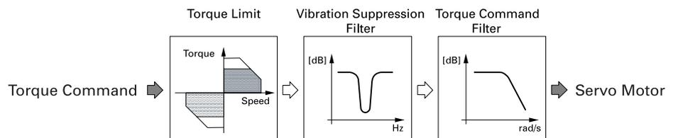
Vibration suppression filter restrains the vibration caused by the load's resonance when the load system resonates in a certain frequency band. If properly set, it allows other gains to be raised, so that the stability and response of the overall system are improved greatly. But if it is set incorrectly, it can cause vibration or noise.
