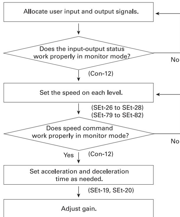
**Multi-level Speed Control Set-up Sequence**
