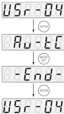
Auto adjustment for torque command offset can be done when the servo is either ON or OFF.
