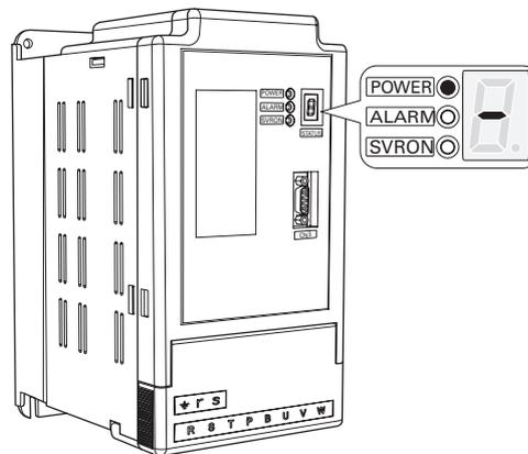
When the power is ON, the middle line will be lit. And the power light will be on.
