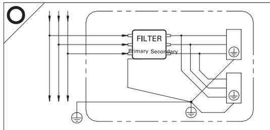
If the noise filter is inside the case, connect the grounding line of the noise filter and all other grounding lines of different devices to the grounding frame and finish the grounding.
