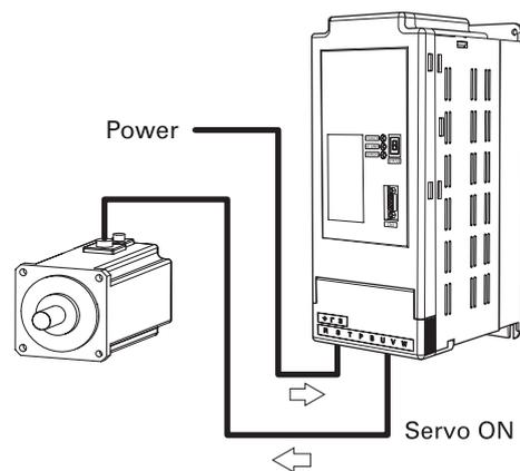
When the controller issues a servo-ON signal, the drive transmits voltage to the motor.
