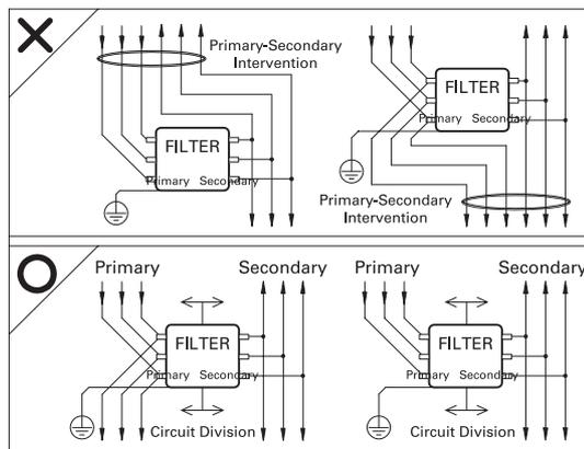
Please separate the input and output wires of the filter, and do not tie them together.
