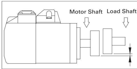
If the center of the shaft does not match, it will lower the performance.
