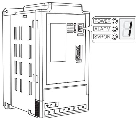
In case of a servo alarm, the LED of the servo drive will display the first number of the relevant alarm code.
