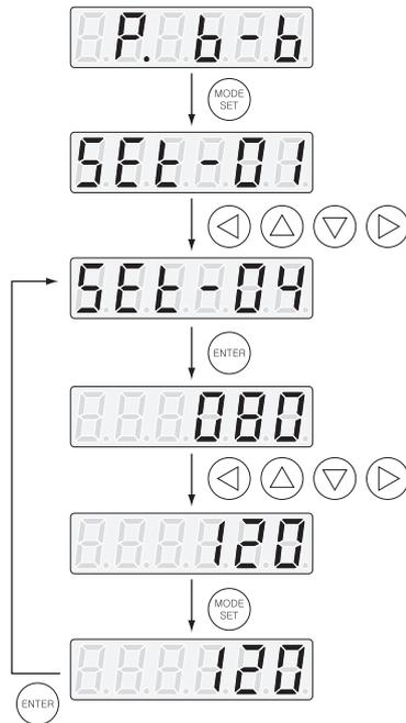
Please press the MODE key until SEt-01 appears. When you see SEt-01, press the direction keys until you see Set-04, the parameter for the position regulator loop proportional gain. Then press the ENTER key and the position proportional gain parameter will be displayed. Press the direction keys to get the value you want and press the SET key to save it. Press the ENTER key to escape from the current level.
