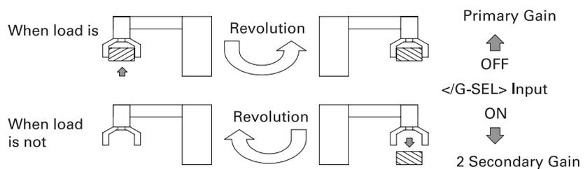
If all the different load conditions are categorized into two, the primary gains and the secondary gains, the response of different load conditions can be satisfied.
