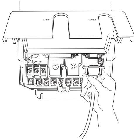
Connect the encoder cable to CN2 connector.
