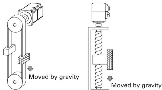
The drive cannot use voltage and current high enough to control the motor brake directly. Therefore, the motor brake cannot be directly connected to the drive. It can be controlled indirectly by building an external circuit through a relay.
