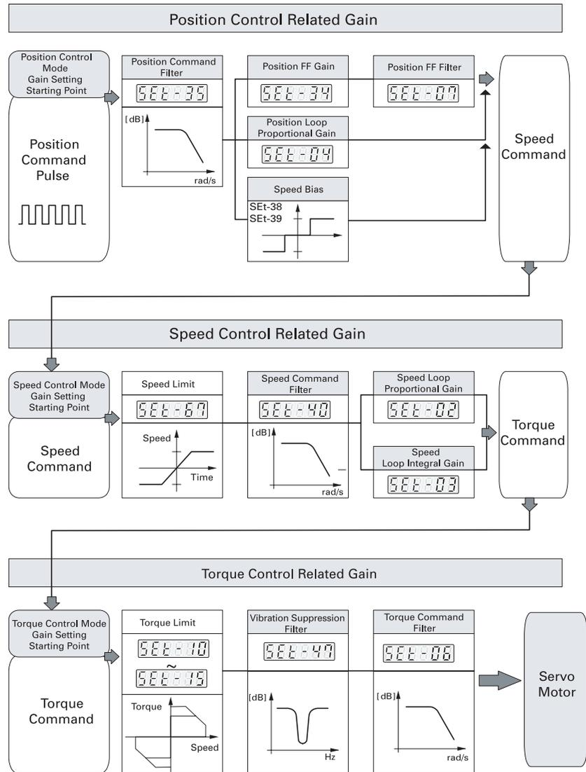
If position-related gains alone are adjusted when the response is not secured enough through setting the gains related to speed control, the system can be unstable. To improve the response of the overall position control system, please secure ample response of the speed control loop.
