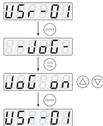
The revolution will continue in the forward direction (counterclockwise) only while the up button is pushed, and in the reverse direction (clockwise) only while the down button is pushed.
