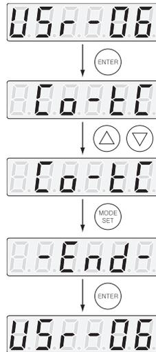
Manual adjustment for torque command offset can be done when the servo is ON.
