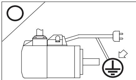
Please connect the grounding line to the grounding connection terminal of the drive.
