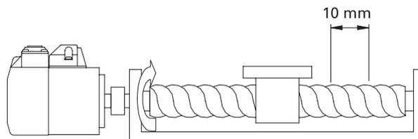
The ball screw finishes one revolution with 1000 pulses and thus a ball screw with 10 mm pitch can move 10 with one pulse command.
