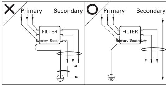
Please position the grounding line of the noise filter away from the output wiring and do not tie it with other signal lines in the same duct.
