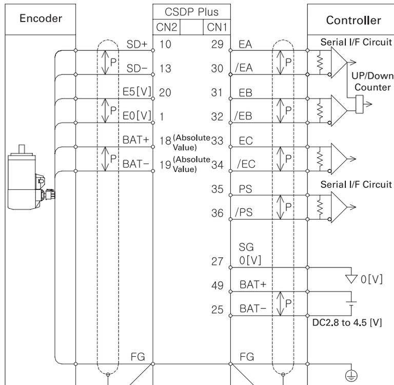
**Serial Encoder Wiring**
